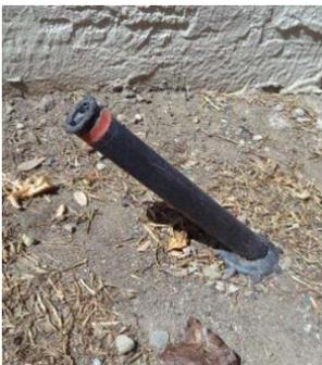
Damaged sprinkler heads are a frequent site in Contempo, costing the Association \$1000's every year. The repair of each sprinkler head is approximately \$70, plus the cost of water lost to leaks. If you see a sprinkler head up after the watering cycle, please gently push or tap the sprinkler head down. Do not kick sprinkler heads.
